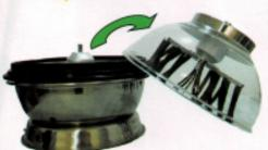
Remove the top from the flower trimmer's base. The inside of the top contains the high-density rubber tongues that are used to push the plant leaves into the blade grill. The cutting blades or wires are located below the grill.
