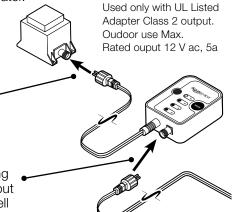
This timer features easy, single-button programming, durable weatherproof construction, and quick-connect weatherproof connections.
