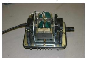
6) Repair only one diaphragm at a time. Remove the black J-tube from diaphragm outlet. Once removed, just push the top of tube to the side out of the way.
