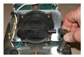
7) Use a Phillips screw driver and remove the 4 screws which connect the diaphragm to the motor plate. You might have to use a flat head screw driver to separate the two halves of the diaphragm.
