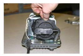
13) Screw the 4 screws in just a little at a time while gradually increasing the torque. Progress around the screws gradually tightening evenly until both halves are fully connected and tight with the motor plate.
