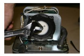
12) Again, properly align the hard plastic with the motor plate. Be sure it is set flush with the motor plate and the oval plug is aligned with hole in motor plate. Now, align the second outer half diaphragm with the first half screw holes. Squeeze both halves together with your fingers really hard. The two halves will not completely connect until you screw them together.
